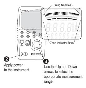
Tuning is shown on the display using tuning needles and zone indicator bars. The tuning needles (at the top of the display) are now zoomed in to enhance laser tuning. For detailed information about Tuning mode, refer to the *FieldMaxII-P User Manual*.
