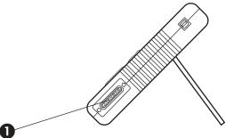
Connect a pyroelectric sensor to the FieldMaxII-P 25-pin connector. *Note: If your sensor has a BNC plug, you will need to attach a 25-pin adapter.*
