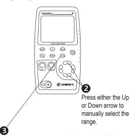
Adjust the trigger threshold from 2 to 20% of range. Make sure the trigger threshold is set below the energy you plan to measure.
